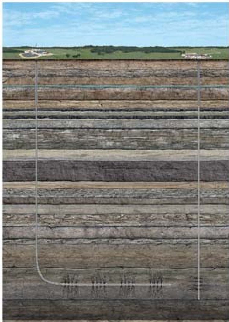
Figure 4: Horizontal and Vertical Well Completions Source: John Perez, Copyright ©, 2008
