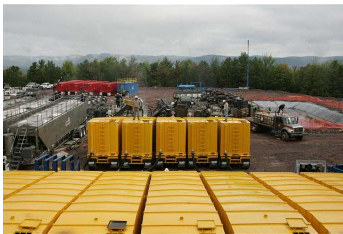
Closed system hydraulic fracturing of a vertical well (PA) Source: ALL Consulting, September 2008
